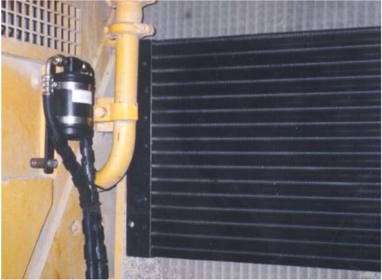
Left side of condenser with drier and hoses in place. Note spacer behind drier bracket.
